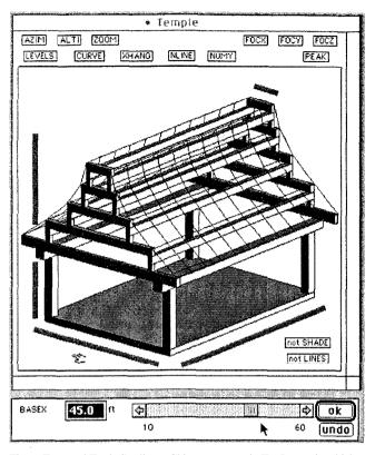
Fig. 6. Toys and Tools Studio. A Chinese Temple in TopDown, in which a designer can manipulate parameters such as the width, length, roof pitch, and different structure of the timber construction.
